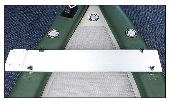
Each FSK16 is hand made so D-ring spacing for each boat is a little different. You may have to push the board back and forth to get the last two bolts through their holes.
