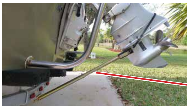
Transom Saver keeps the motor secured at an angle.
