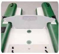
Motor Mount Transom Board Insert transom board into motormount grommets. Plate with ring faces forward.
