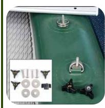
Near valves in bow (front) are four D-rings (two on each side of boat) that hold the aluminum board to the boat.
