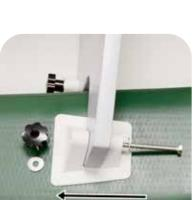
Push the 100mm (4") x M8 bolts with washer through the grommets and transom. If needed, push sides so transom holes align with grommet holes. A wrench is recommended for holding the bolt heads while tightening the threaded knob. When all four bolts are inserted, inflate the side chambers to the working pressure.
