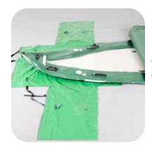
When all the air is pushed out. Place the boat bag under the bow.
